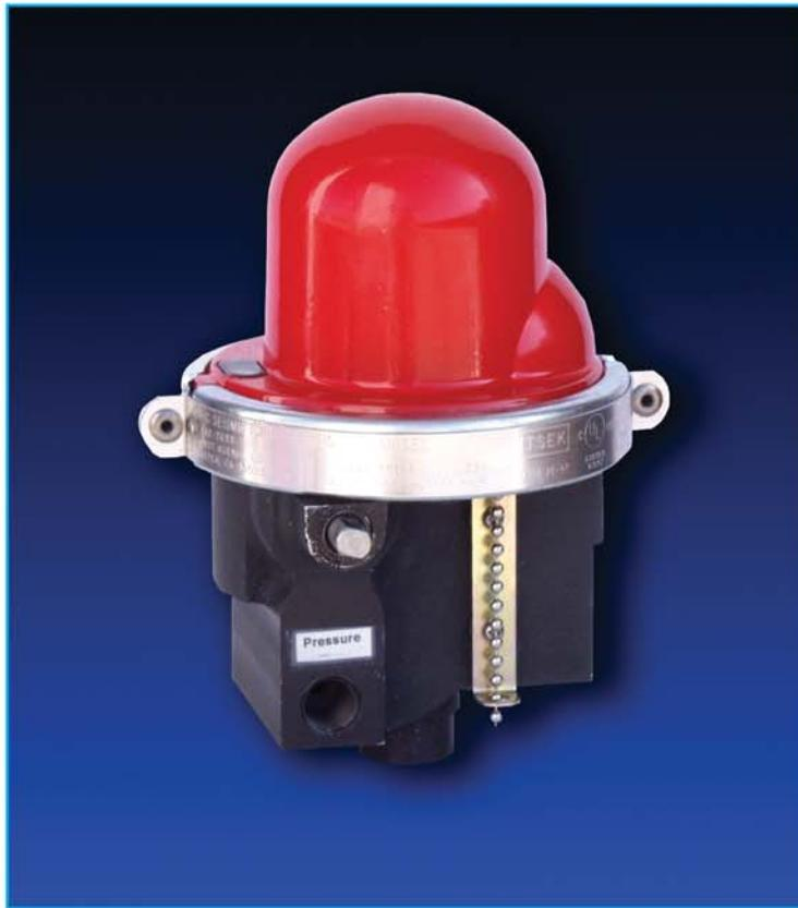
The Model 400 earthquake actuated 3 way valve offers a redirection of dry air or nitrogen from the pressure ( n/o ) to the exhaust ( n/c ) port during a seismic event. Reset is simple using a flat blade screw driver and the valve status window, see included instructions.
