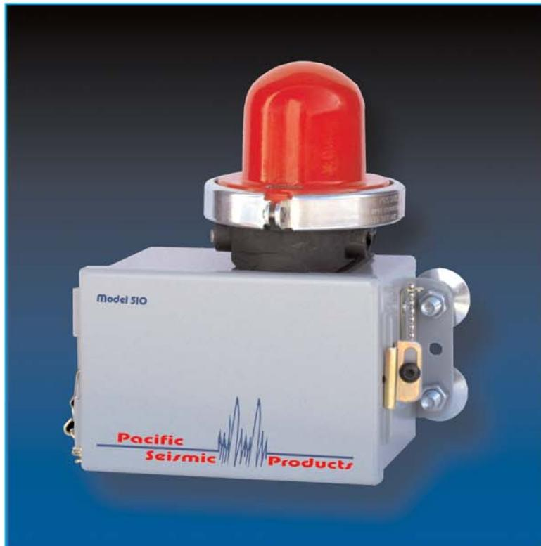
The Model ES510 Seismic Switch is a seismically actuated electrical switch. This unique device, when configured properly, will cut electrical power to just about any device during a seismic event. It is mounted securely to the building via mounting brackets and leveled using chain site. The protected device's power is wired with the 510 and other customer provided hardware thus providing seismic protection.
