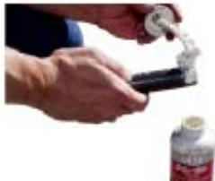
8. Use teflon tape or liquid sealant on all joints.
