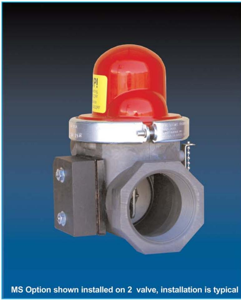
The new Model MS Monitoring Switch is an optional feature that is available at the time of order with any CALIFORNIA valve. This unique device relays an electrical signal that enables the valve's open or closed position to be monitored remotely. It is mounted by the factory on the side of the valve, and does not interfere with the position-indicator window with the green and red tags.
